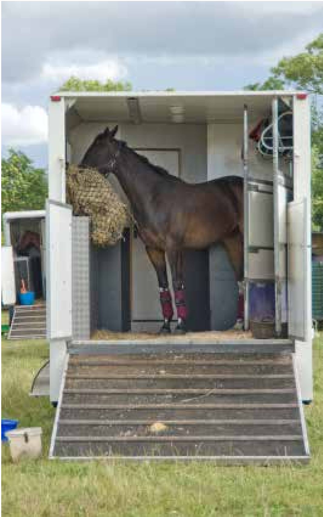
Horse trailers and vans must have sufficient height to allow horses to stand fully upright and must allow sufficient space for each horse. Doors and ramps should be sufficiently wide to provide safe loading and unloading.
